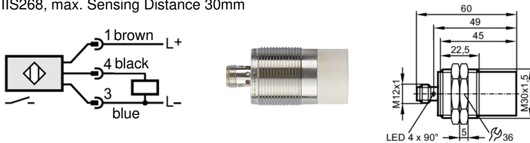
Fig. 5.5.3 Typically used proximity sensor as Rotation Sensor IIS268, max. Sensing Distance 30mm
