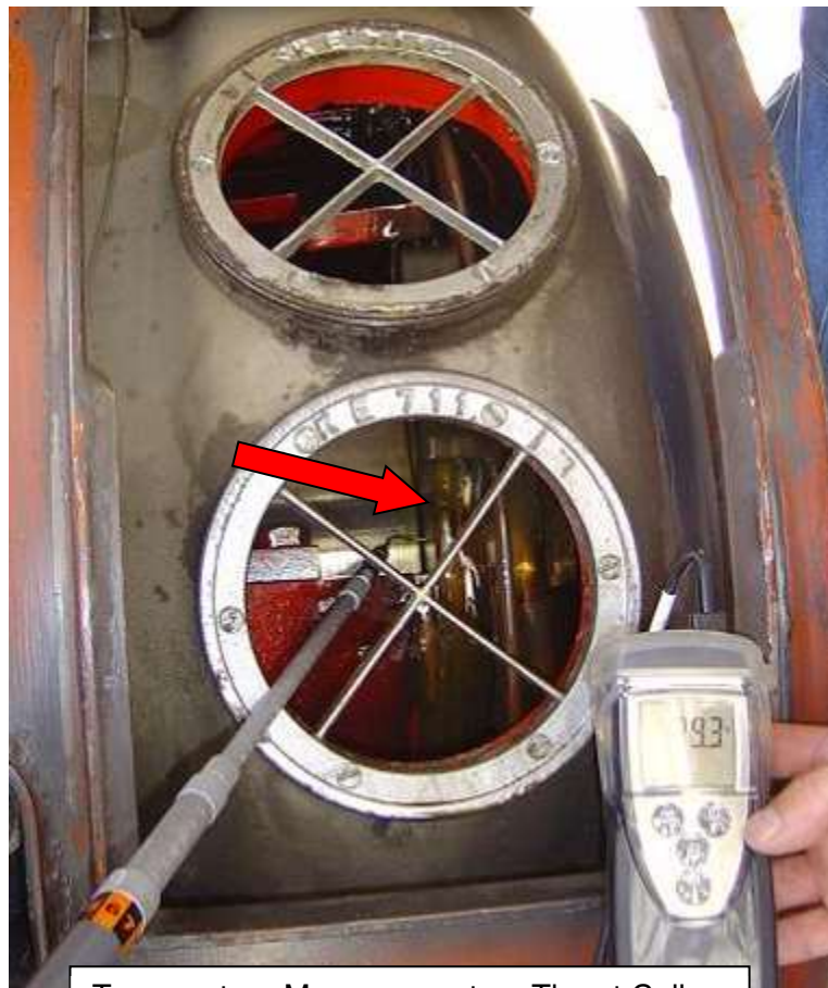
Temperature Measurement on Thrust Collar
