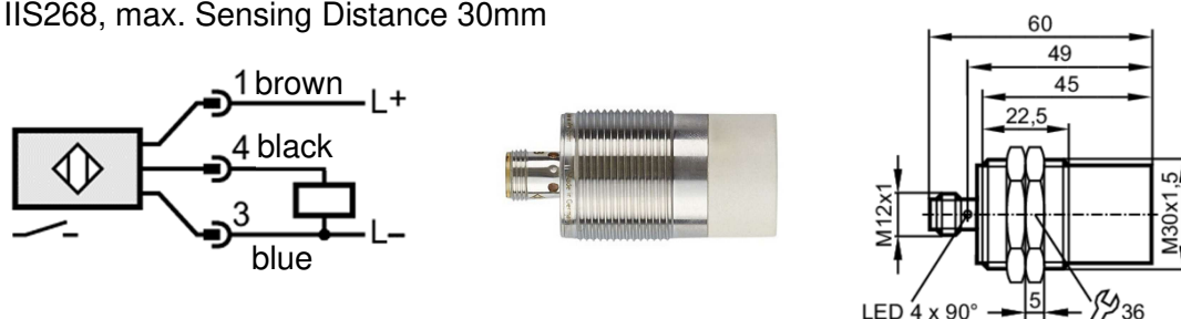
Fig. 7.6.3 Typically used proximity sensor as Rotation Sensor IIS268, max. Sensing Distance 30mm
