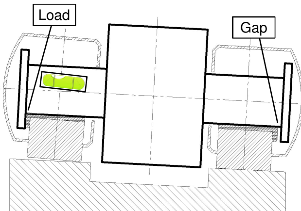
Fig. 4.1.1 Thrust Disc is attached to the shaft end
