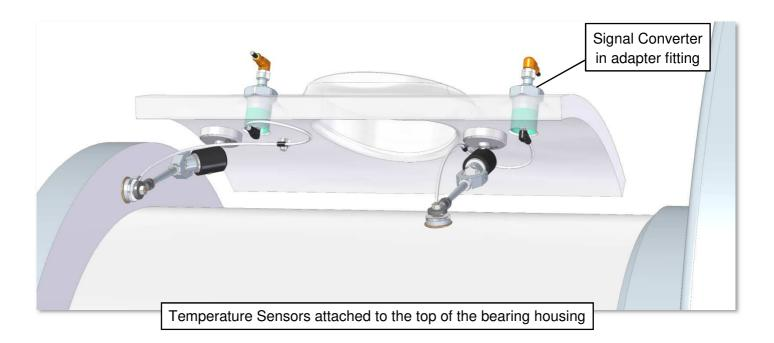
Some bearing housing allow only access from the top through the inspection door. The magnetic stand can be attached from top as well.
