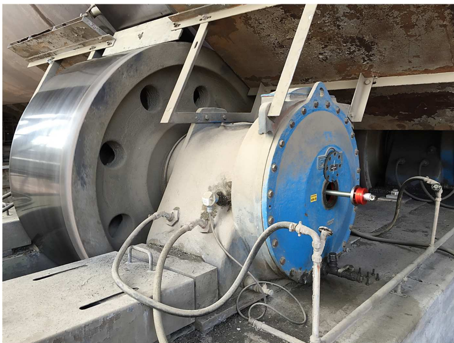
Fig.10.1.2 Ball prism attached to the roller shaft
