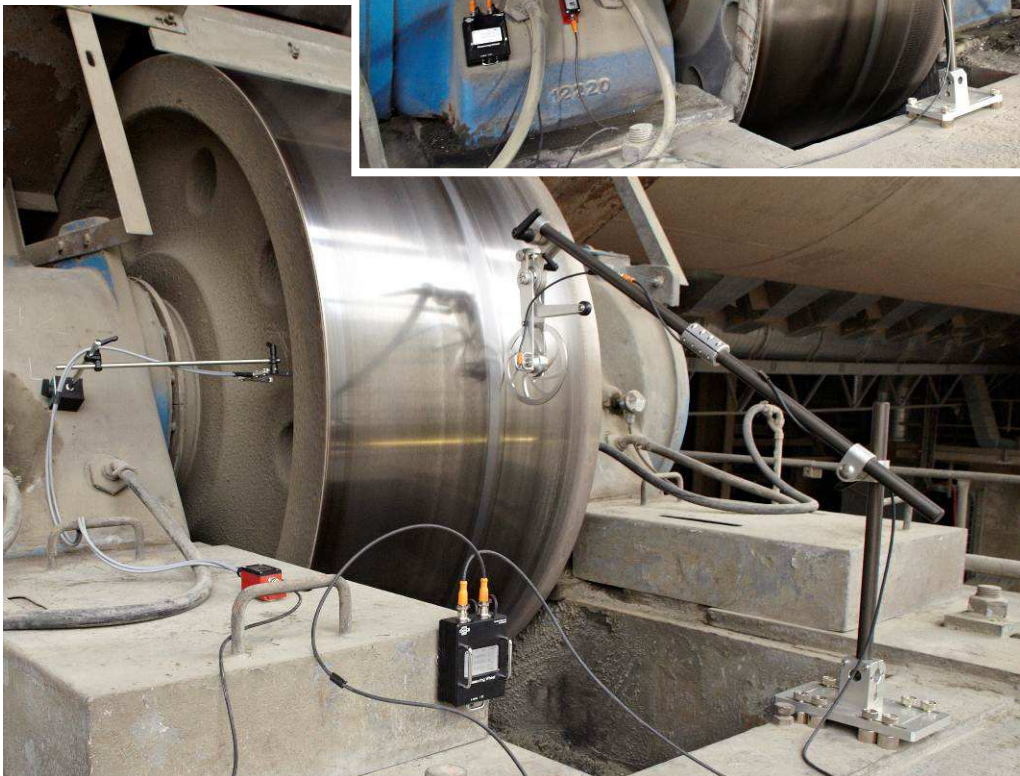
Measurement of support roller diameter
