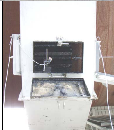
Measurement of Girth Gear Run-Out
