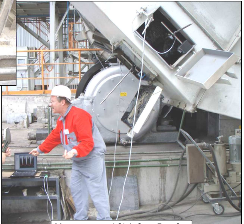
Measurement of Girth Gear Run-Out
