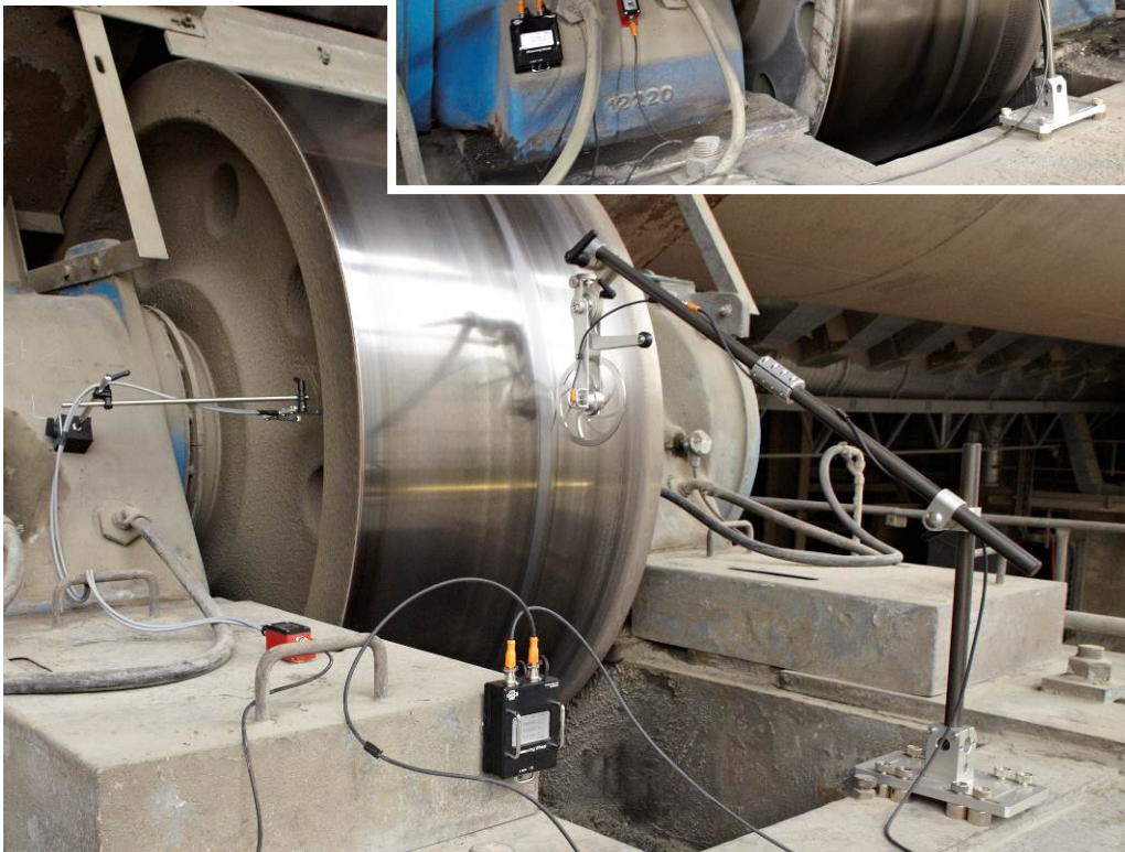
Measurement of support roller diameter
