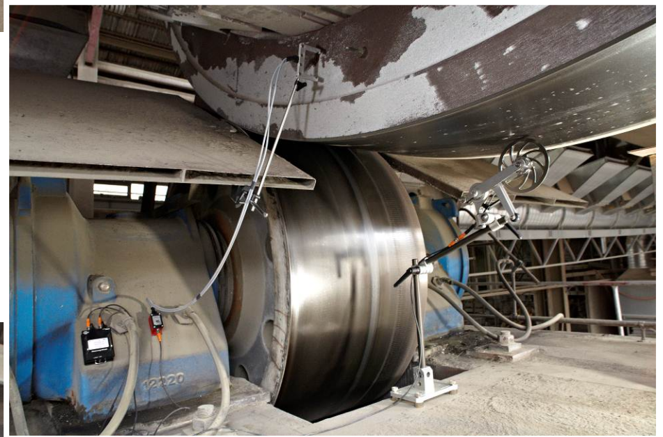
Measurement of kiln tire diameter
