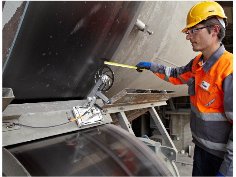
Measurement of kiln tire diameter
